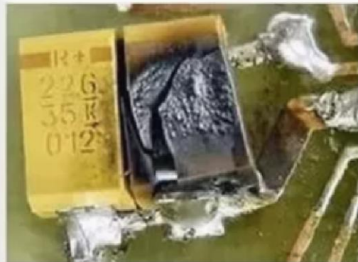
tantalum capacitors can "go up in smoke"
